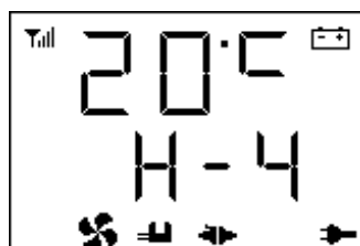
start-up mode, manual mode (marked with H)
