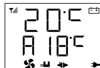
start-up mode, automatic mode (marked with A)
