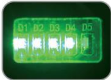
Battery capacity indicator Each LED indicates 20% battery charge.
