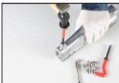
5. Using a tip break tool, break off the adapter mount.
