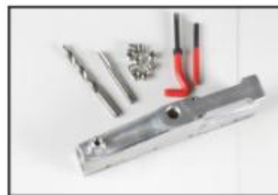
6. The thread is repaired and ready for use.
