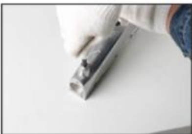
4. Screw the adapter into the threaded hole.
