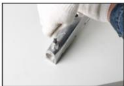
4. Screw the adapter into the threaded hole.
